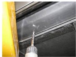
11. There are 2 additional holes in the side skirt. Drill through these holes using a 1/8" drill bit, then attach the provided self-tapping screws.
