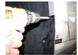
10. There are 2 additional holes in the rear wheel well extension. Drill through these holes using a 1/8" drill bit, then attach the provided self-tapping screws.
