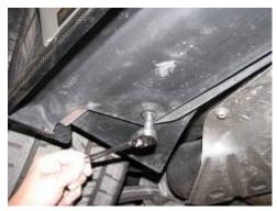
5. Attach the side skirt using the original bolts that were removed (3 at the front, 1 at the rear).
