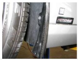
3. Remove 1 bolt in the rear wheel well just ahead of the rear tire, then attach the wheel well extension using the original bolt.
