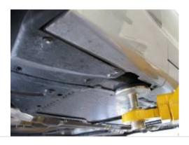
1. Remove 3 bolts from the bottom of the front fender, just ahead of the door.
