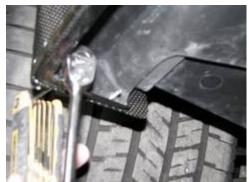
6. Align the wheel well extension to the side skirt, then secure using the provided bolts, nuts, and washers.
