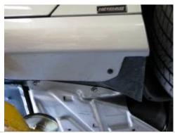
2. Remove 1 bolt from the bottom just behind the door.
