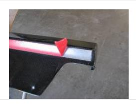
4. Peel away a small portion of the adhesive backing tape at the rear of the side skirt.
